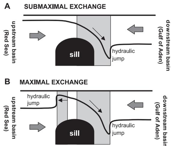
Fig. 3. Hydraulic exchange regimes for two-layer flow as explained in the text. Large grey arrows represent the fluxes in each layer. Grey regions represent supercritical flow where changes to the interface are swept in the direction of the small black arrows.
