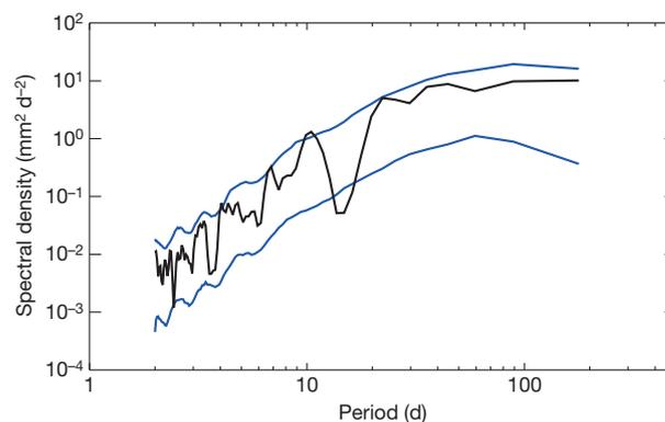
**Figure 2 | Power spectra of daily river runoff for England and Wales autumns.** Black line shows the spectrum for runoff synthesized from ERA-40 precipitation in all available autumns (1958–2001). Pair of blue lines marks the 5–95% confidence interval of the spectrum for runoff synthesized from all precipitation simulations in the A2000 climate.
