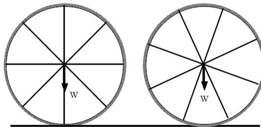
We start by using only 8 beam elements (1 per 45° sector) and we calculate the downward displacement of the center of the wheel towards the floor and the maximum spoke tensile and compressive stresses (unit?).
