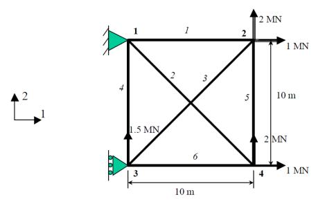
Figure 1. Truss structure
