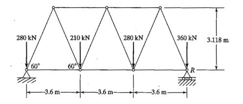
Analyze this railroad bridge problem by using ABAQUS. Find out the nodal displacements and element stresses for every node and element, including the horizontal displacement of point R. The railroad bridge is made from steel and has a Young's modulus of 210 GPa.
