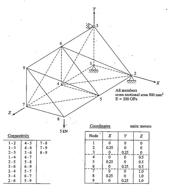
Find out the nodal displacements and element stresses for every node and element. (Hint: 3D truss element is T3D2).
