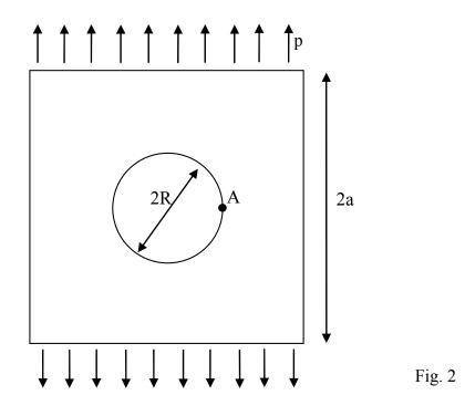
Use 3-node triangular elements to solve the classic stress concentration problem in ABAQUS/CAE. A small circular hole with radius R is in the middle of a square sheet (with width 2a). A uniform tension p is applied on the top and bottom surfaces of the sheet. The problem can be taken as plane stress. You may only mesh 1/4 of the model by using the 2-fold symmetry conditions.
