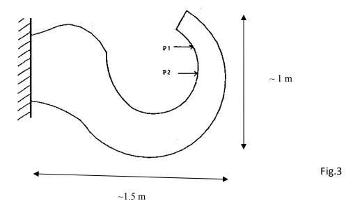
Analyze the metal hook shown in Fig. 3 in which the geometry, loads and boundary conditions are also indicated. The problem can be taken as plane stress. The hook is loaded by two concentrated forces, P1 and P2, each of a magnitude of 25 kN. The material is assumed to be elastic and isotropic with an elasticity modulus E=210GPa and Poisson's ratio v=0.3.
