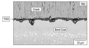
Fig. 1. TGO undulations in a thermally cycled system with a yttriastabilized zirconia top coat and a Pt aluminide bond coat [3].
