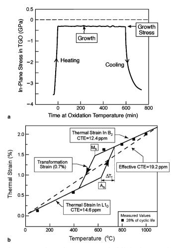
Fig. 3. (a) Growth stress in a TGO on a Pt aluminide bond coat [15]. (b) Martensite transformation in a Pt aluminide bond coat [19].
