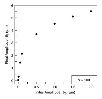
Fig. 7. Variation of the final undulation amplitude with initial amplitude.
