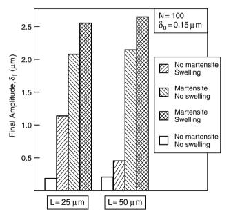
Fig. 8. Comparison of final undulation amplitude with and without swelling and martensite. Results are shown for two wavelengths.
