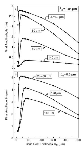
Fig. 6. Variation of the final undulation amplitude with bond coat thickness, for various initial undulation shapes, as predicted by the model with a finite thickness substrate. Swelling is not included.
