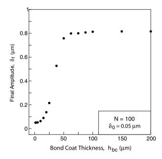
Fig. 5. Variation of the final undulation amplitude with bond coat thickness as predicted by the model with an infinitely deep substrate.
