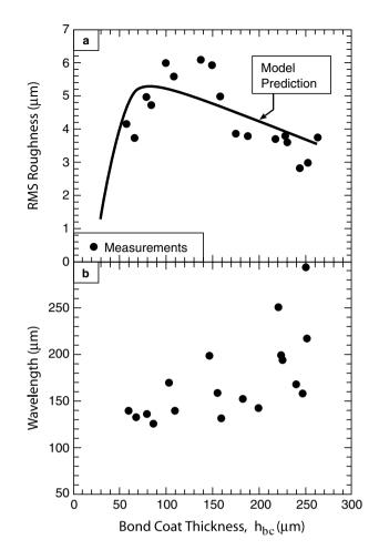
Fig. 2. Experimental observation that the rumpling rate of a Pt aluminide bond coat depends on its thickness [12]. The simulation result is superposed.
