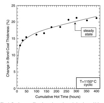
Fig. 4. Bond coat swelling observed as a change in bond coat thickness with high-temperature exposure [13].
