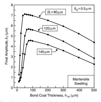
Fig. 9. Variation of the final undulation amplitude with bond coat thickness, for various initial undulation shapes, as predicted by the model with a finite thickness substrate. Swelling is included.
