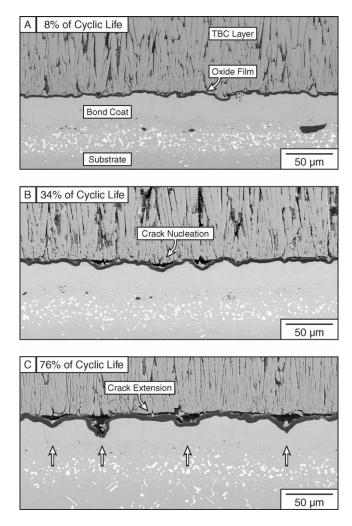
Fig. 2. An example of the displacements of the TGO that accompany thermal cycling of a thermal barrier system with a Pt-aluminide bond coat (courtesy D.R. Mumm). The arrows identify the instability sites. Note the downward displacement of the TGO layer into the bond coat as the fraction of life (indicated as percentages) increases from (a) to (c).
