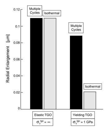
Fig. 10. Simulations comparing the radial enlargement for isothermal and cyclic conditions, for an elastic TGO ( $\sigma_{\rm Y}^{\rm tgo}=\infty$ ) and a yielding TGO ( $\sigma_{\rm Y}^{\rm tgo}=1$  GPa),  $\sigma_{\rm Y}^{\rm bc}=200$  MPa, N=24,  $\Delta\varepsilon_{\rm g}=10^{-3}$ . Absent yielding, the same radial change occurs for isothermal and cyclic conditions.
