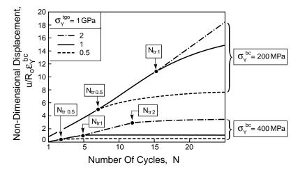
Fig. 15. The cycle-by-cycle development of the non-dimensional radial enlargement for various TGO yield strengths. When TGO yielding occurs,  $N_{\rm cr}$  a steady-state is reached wherein the enlargement is caused entirely by the thickening of the TGO.
