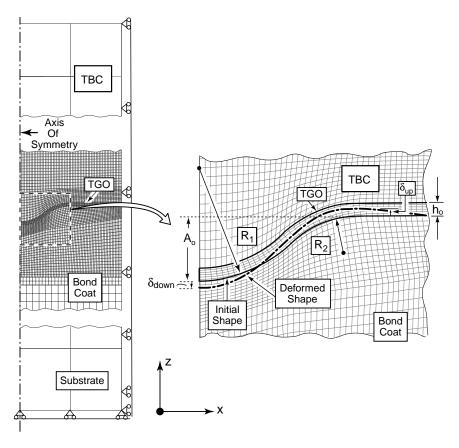
Fig. 3. Example of finite element model previously used to simulate the displacements in Fig. 2 (Karlsson et al., 2002b). The shape of the imperfection is varied by changing the ratio between the two characteristic radii  $R_2/R_1$ .
