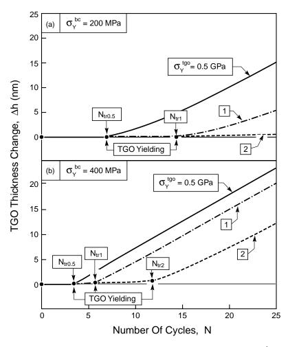
Fig. 16. The cycle-by-cycle thickening of the TGO for various TGO yield strengths: (a)  $\sigma_{\rm Y}^{\rm bc}=200\,{\rm MPa}$  (b)  $\sigma_{\rm Y}^{\rm bc}=400\,{\rm MPa}$ . When TGO yielding occurs, the TGO thickness increases, even though the imposed thickening strain is zero.
