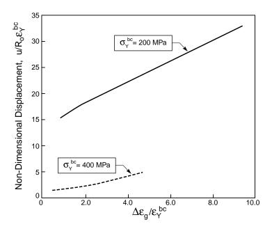
Fig. 13. Numerical simulations showing that the radial enlargement increases with increasing incremental growth strain (after 24 cycles,  $\sigma_y^{tgo} = 1$  GPa).
