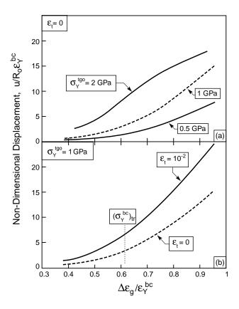
Fig. 14. The non-dimensional radial enlargement (N=24) as an inverse function of bond coat yield strain (for growth strain  $\Delta \varepsilon_g = 10^{-3}$ ). (a) Larger TGO yield strength results in smaller displacements. (b) Including a thickening growth strain leads to larger displacements but similar trends.
