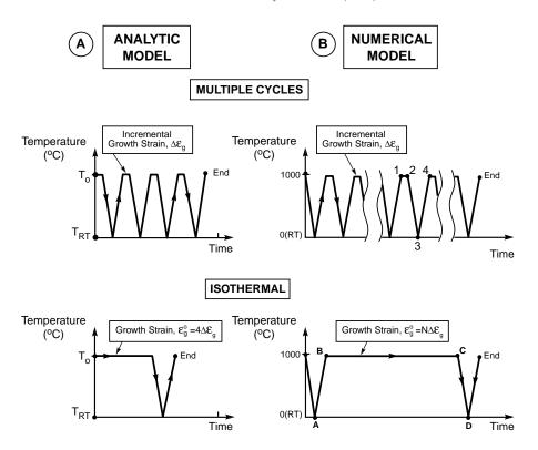
Fig. 7. The two thermal histories used to conduct calculations with the analytical and numerical models.
